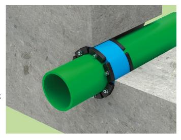
Pressio Blue (Type BC and BS) molded links have a softer durometer (40  $\pm$  5 Shore A) for thinner wall pipe application. Also used for larger model sizes for engineered rubber expansion for better bolting performance.
